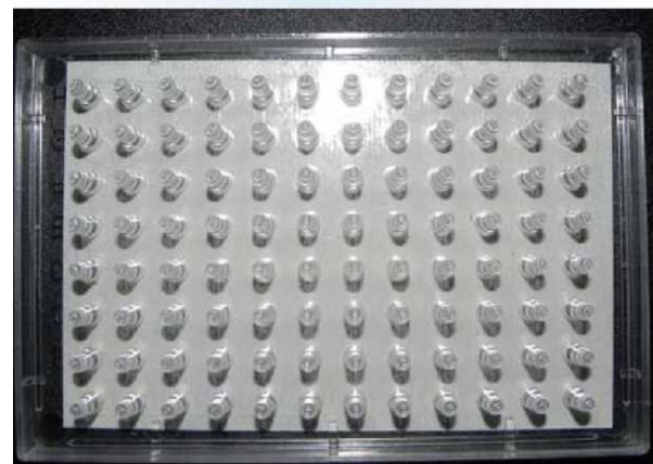
FIGURE 2.34 Biofilm detection micro-well plate (MBECTM-Device). The MBECTM-Device has 96 removable pegs (adhesion medium) in its plate cover that sit in the 96 micro wells in the corresponding base. Biofilm formation on the 96 pegs can be detected at the same time, but every peg can also be removed when the biofilm on that peg must be analyzed independently.
